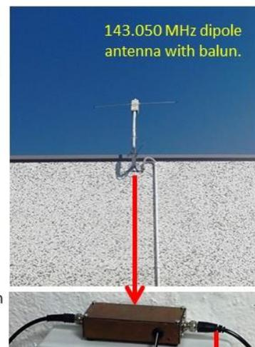
Antenna LNA with 143.050 MHz band-pass filter.
