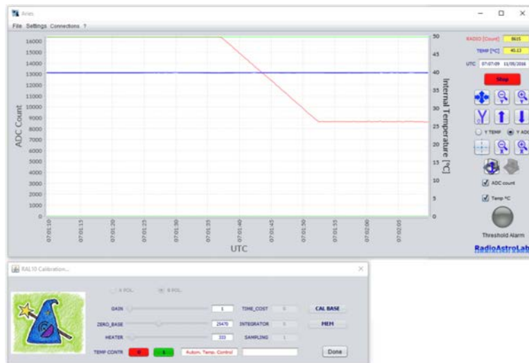
FIGURE 3.11: The radiometric signal (red track) is stable in the middle of the acquisition scale after the baseline calibration.
