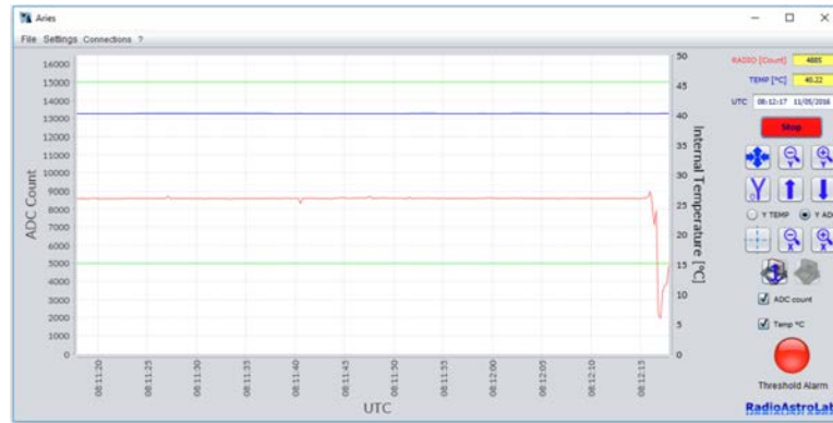
FIGURE 4.11: Alarm that alerts when the radiometric signal goes over the values of the pre-set thresholds (green horizontal lines on the graphic window).
